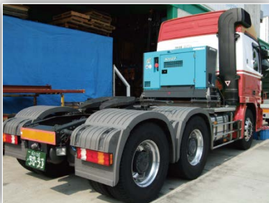
Cabin Back Loading
